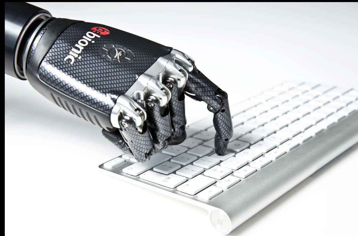
The four primary control signals used by myoelectric prosthetics allow movements such as flexion and extension of the elbow and hand.
