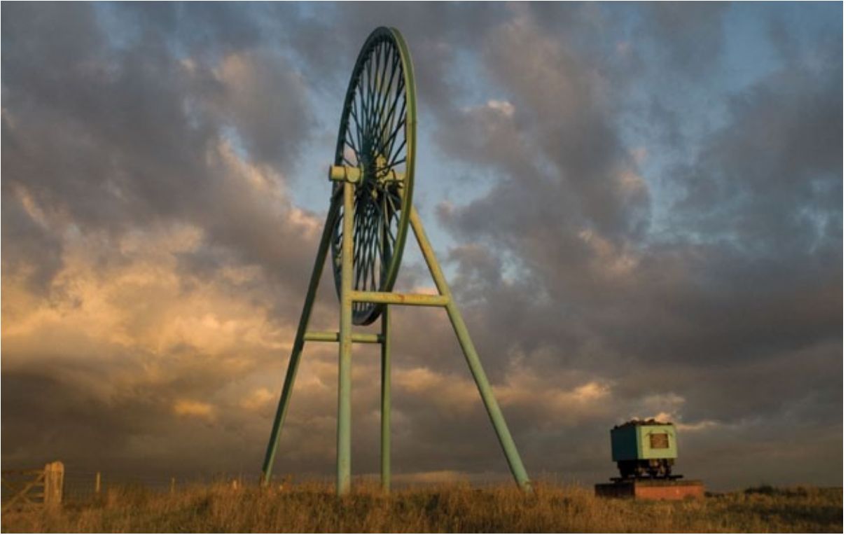
A powerful US coal lobby: this winding wheel controlled cages to take men to and from the bottom of the mine
