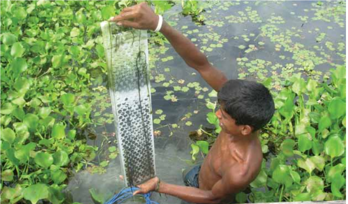
In a flooded paddy, a boy from Bashaibhog village, Bangladesh helps to collect porewater samples from various sediment depths where arsenic contamination levels are typically around 400 ppb and can be up to 2500 ppb
